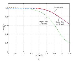
Aliasing errors tend to restrict the application of the invariant impulse-response method to the design of allpole filters, i.e., filters that have no zeros in the finite s plane.
