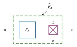
• On the basis of the Poisson summation formula (see Chap. 6), the impulse-modulated filter can be represented by a continuous-time transfer function  $\hat{H}_A(s)$  or, equivalently, by a discrete-time transfer function  $H_D(z)$  as follows:
