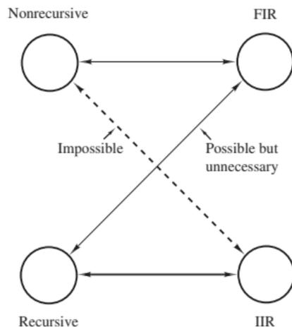
**Note:** An IIR system *cannot* be a nonrecursive system and vice-versa. However, a recursive system can be constructed that is also an FIR system but such a system would serve no useful purpose.
